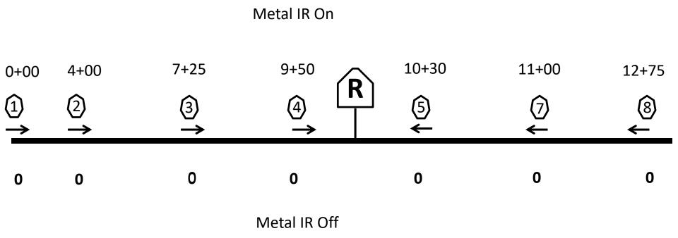
In the On the current is flowing to the negative return connection of the rectifier In the off the pipe is perfectly coated as well as perfectly isolated, no galvanic flow Now put in your +/- Reads from your metal IR On' & Off's (This shows a perfect world scenario - Mag Beds)
