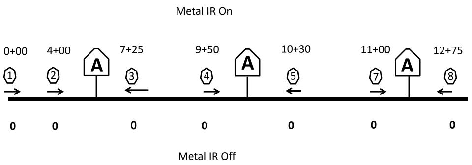
In the On the current is flowing to the negative return connection of the rectifier In the off the pipe is perfectly coated as well as perfectly isolated, no galvanic flow Now put in your +/- Reads from your metal IR On' & Off's (This shows a possible area to investigate - Rectified)
