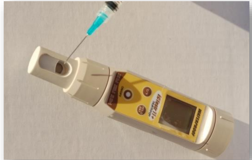
Conductivity Measurement (not ion-specific)
