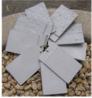
ICRI 310.2R Replica Stamps (For Concrete Surface Profile – CSP)
