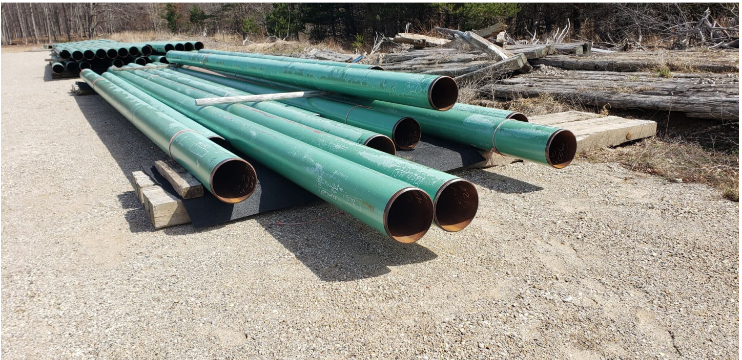
Figure 4-6: Pipe in Yard with Factory Applied FBE
