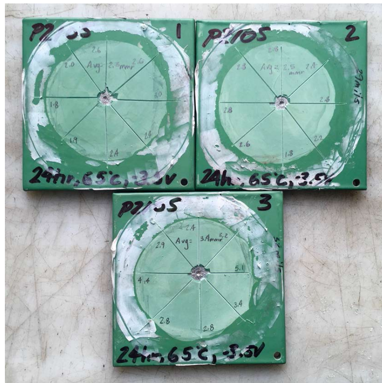
Figure 4-1: Cathodic Disbondment Test at 149°F, 3.5 Volts of Cathodic Protection, and for 24 Hours
