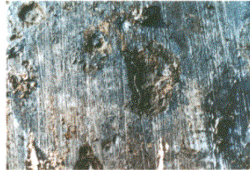
b. Corrosion in pit
