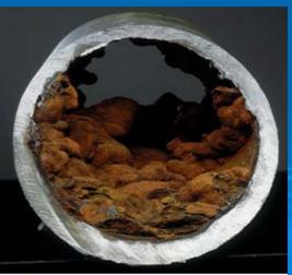
Photo: Extensive tuberculation can discolor and contaminate water as well as result in greatly reduced water flow and pressure.
